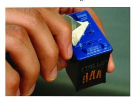
Peel the sticker from one corner using a sharp blade
